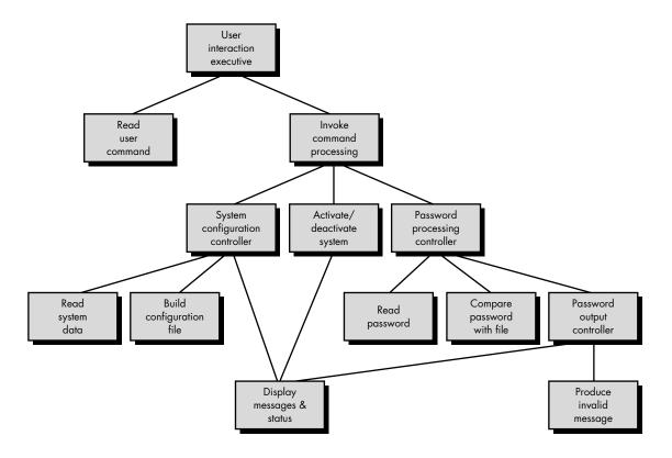
FIGURE 14.16 First-iteration architecture for user interaction subsystem
