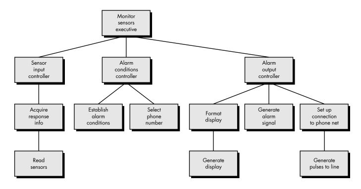
FIGURE 14.11 "First-iteration" program structure for monitor sensors
