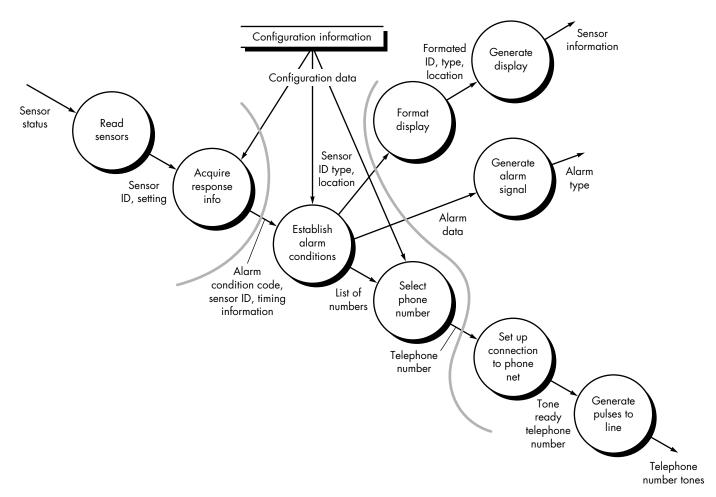
FIGURE 14.8 Level 3 DFD for monitor sensors with flow boundaries
