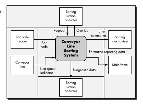
arrows shown in the SCD represent information (data and control) as it moves from the external environment into the CLSS system. The external entity *bar code reader* produces input information that is labeled **bar code**. In essence, the SCD places any system into the context of its external environment.
