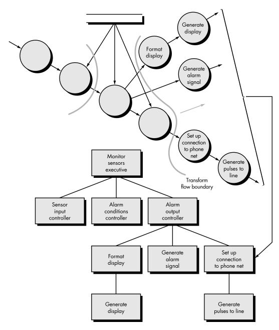
FIGURE 14.10 Second-level factoring for monitor sensors
