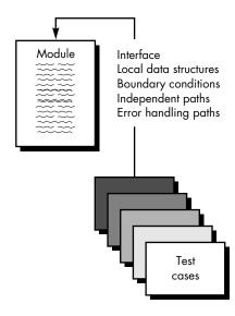
FIGURE 18.4 Unit test Tests of data flow across a module interface are required before any other test is initiated. If data do not enter and exit properly, all other tests are moot. In addition, local data structures should be exercised and the local impact on global data should be ascertained (if possible) during unit testing.
