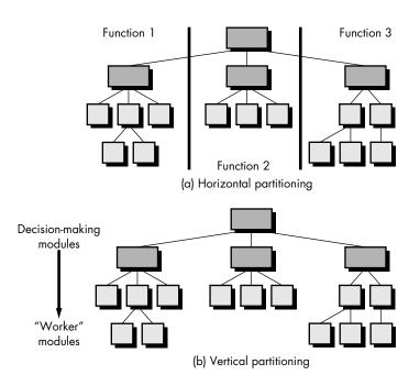
Vertical partitioning (Figure 13.4b), often called *factoring*, suggests that control (decision making) and work should be distributed top-down in the program structure. Top-level modules should perform control functions and do little actual processing work. Modules that reside low in the structure should be the workers, performing all input, computation, and output tasks.
